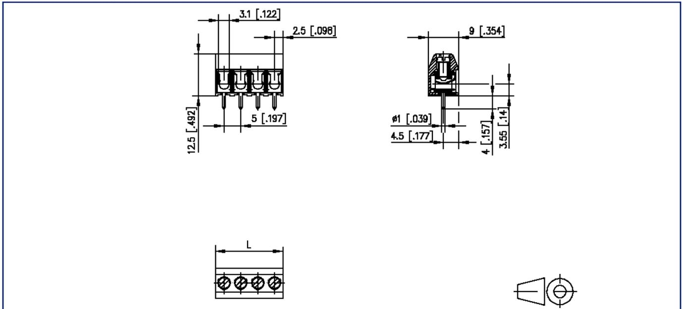
$L = (\text{pole size} - 1) \times \text{centerline} + 5 \text{ mm } [0.197]$
