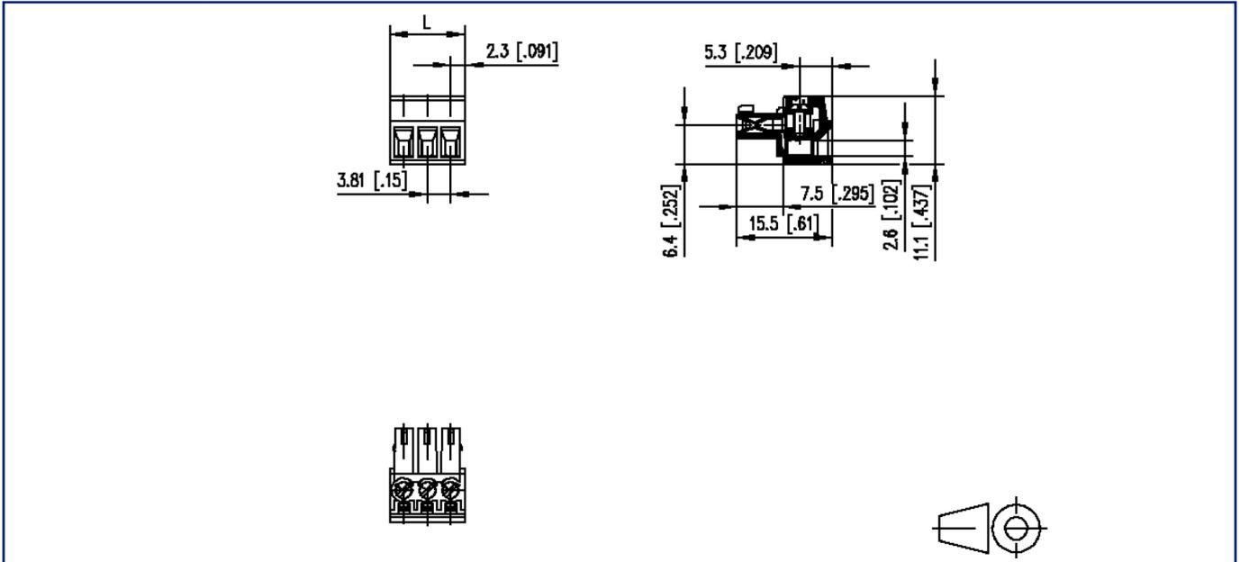
$L = (\text{pole size} - 1) \times \text{centerline} + 4.6 \text{ mm} [0.181]$
