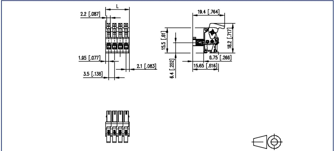
$$L = (\text{pole size} - 1) \times \text{centerline} + 4 \text{ mm } [0.157]$$
