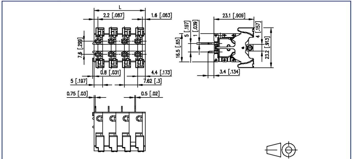
$L = (\text{pole size} - 1) \times \text{centerline} + 6.6 \text{ mm} [0.26]$
