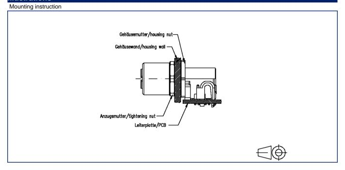
Tightening torque - Jack mounting
